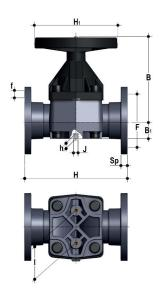
VMOAC Diaphragm valve with flanged monolithic body, drilled ANSI B16.5 cl.150 #FF
